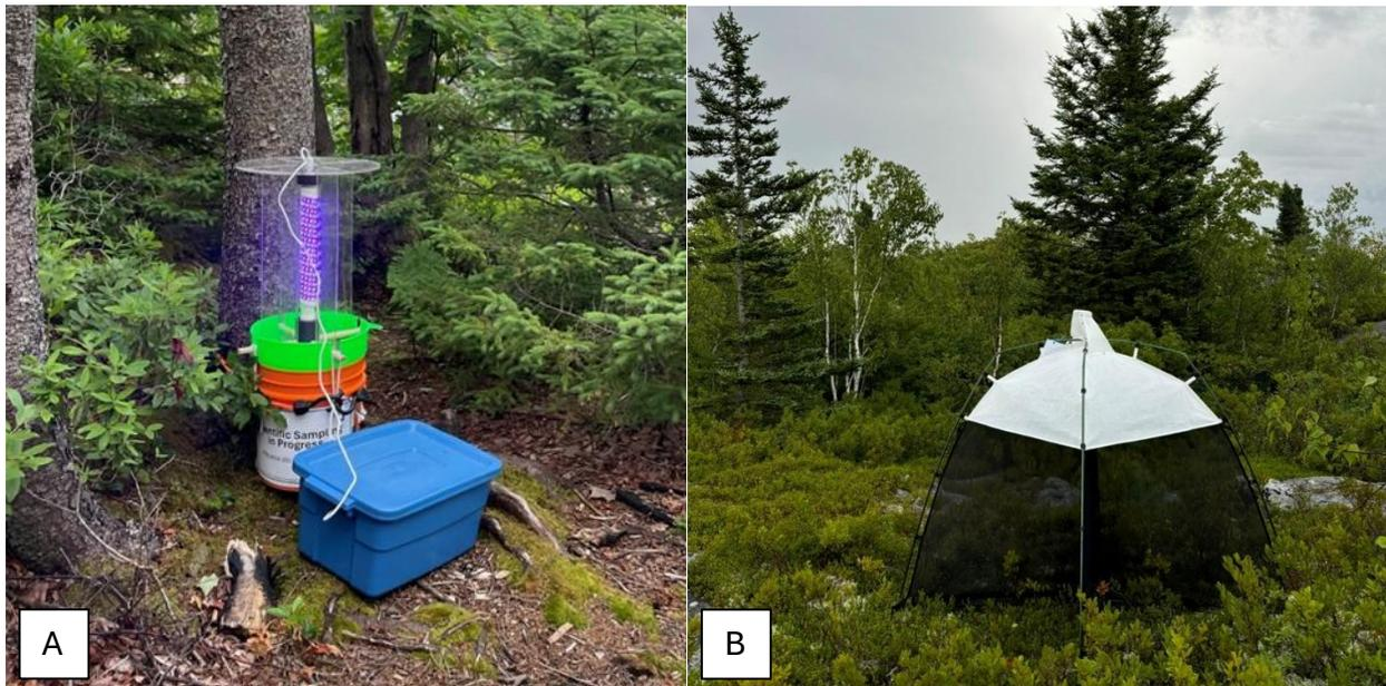
**Figure 2. Sampling equipment.** Shown are the two trap types used for insect collection. A) Light trap design built around the Entolight, an LED light with UV spectrum emissions produced by *Entoquip*. B) SLAM trap II Malaise intercept trap by *BugDorm*.
